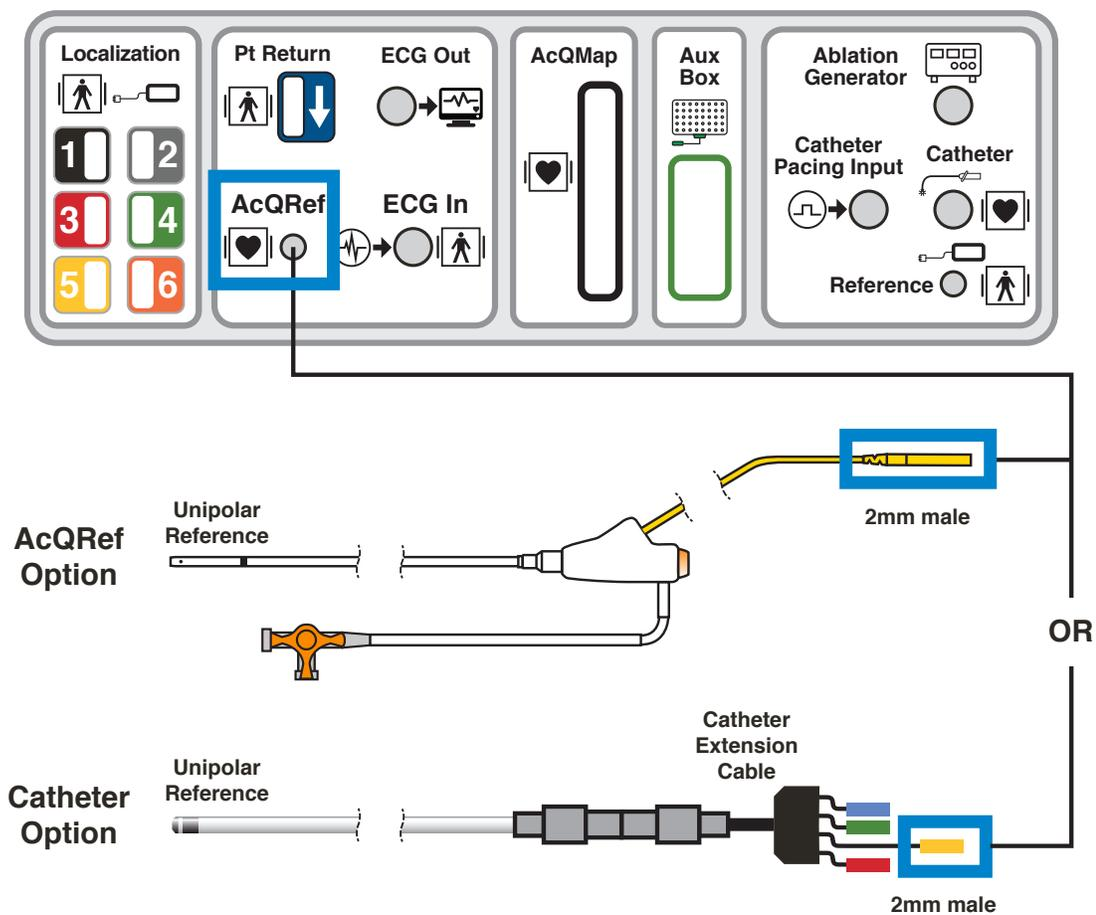
Figure 5-2. Electrical Reference Catheter specifications and connections.
