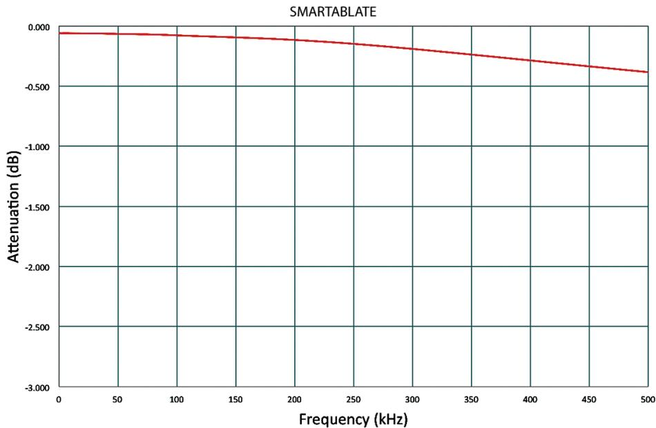
Attenuation of signals using the SMARTABLATE Generator and the AcQMap Console front panel
