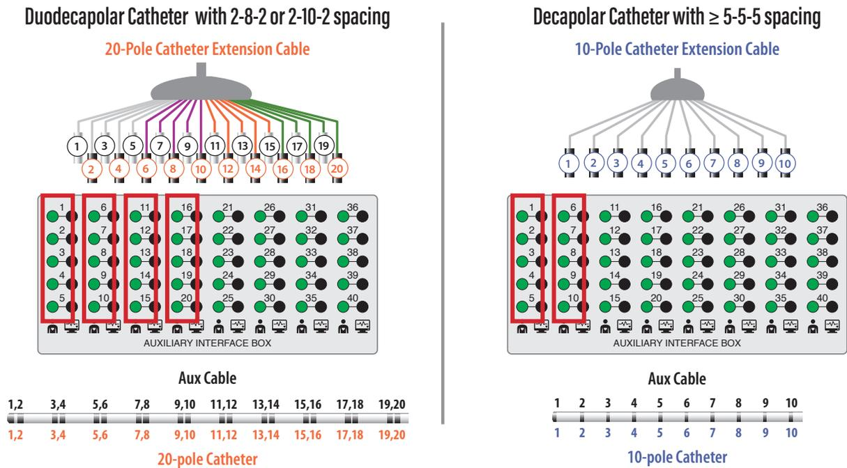
Figure 5-3. Anatomic Reference Catheter specifications and connections.
