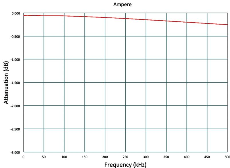
Attenuation of signals using the Ampere Generator and the AcQMap Console front panel
