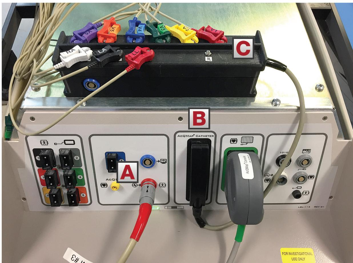
Figure J-1. ECG Cable test connections. (A) ECG Input Cable. (B) ECG POST Cable 80526 is connected to the AcQMap Catheter receptacle on the console front panel. (C) Connect each ECG connector to the corresponding name of ECG lead.
